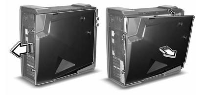
c Lift the panel upward to detach it.
